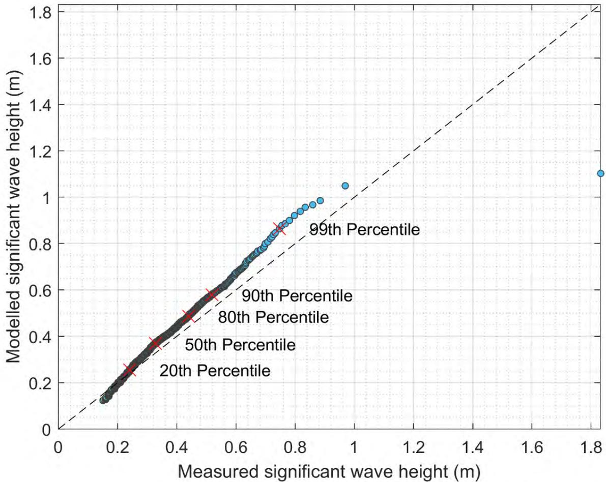
**Figure 39: Calibration (Q\_Q) plots of modelled waves heights against measured wave heights at the Emu Point and Lockyer Shoal AWAC devices (DoT) from the 41-year wave hindcast model.**
