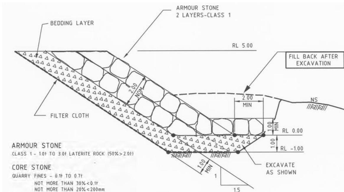
Figure 25: Design profile of Coastal Structure A (sourced from: DoT, 2007)
