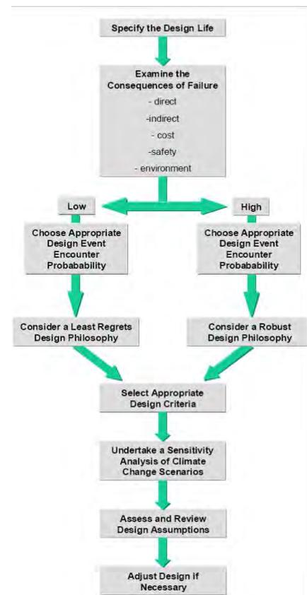
practice for general criteria, BSI 07-2000) and AS 4997-2005 (Guidelines for the design of maritime structures) are widely used for the selection of the most appropriate design event.
