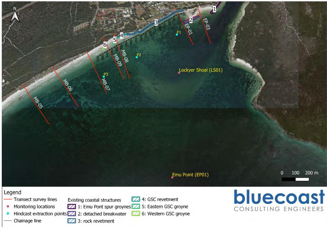
**Figure 40: Emu point monitoring locations and hindcast model extraction location**
