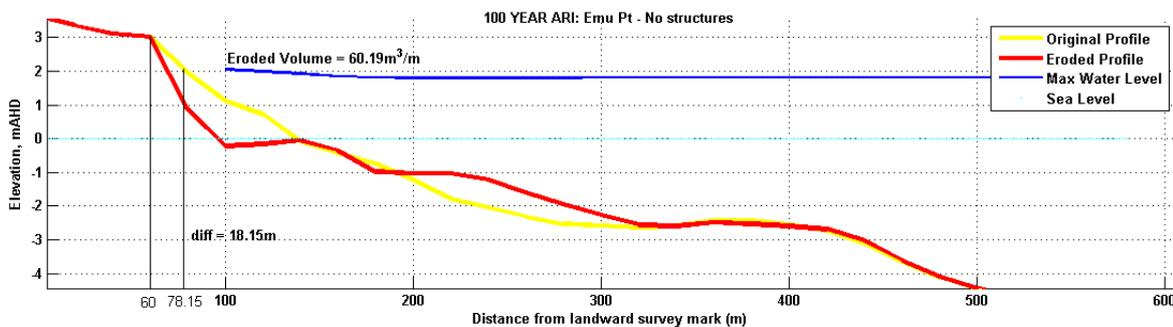
Figure 15 SBEACH storm erosion – 100year ARI at Emu Point (source: RHDHV, 2017).
