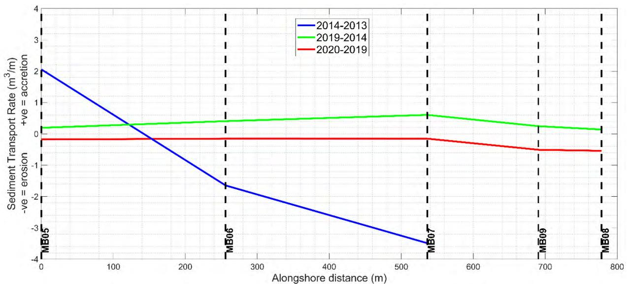
**Figure 54: Sediment transport rates (m<sup>3</sup>/m) between MB-05 and MB-08 for the periods 2013 to 2014, 2014 to 2019 and 2019 to 2020. Note: erosion is negative.**
