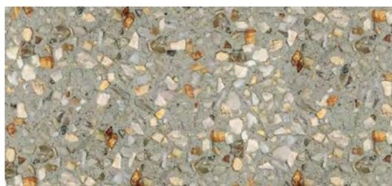
1. Exposed aggregate concrete - Sandstone Pebble
