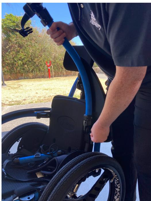
**Step 2.** Lift the armrest up. Lifting the armrest may improve accessibility when transferring the user to the beach wheelchair.
