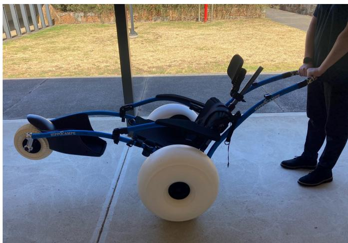
**Step 1.** Lift the front wheel off the ground to turn left or right.
