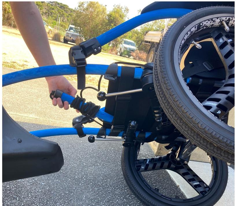
**Step 3.** Place the rope underneath the seat, in the gap between the seat and black straps.
