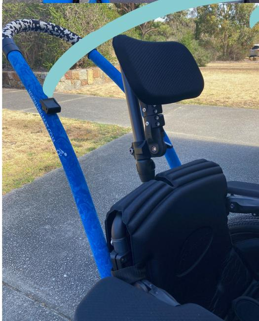
**Step 2.** Lift the black clip attached to the push bar to remove straps.
