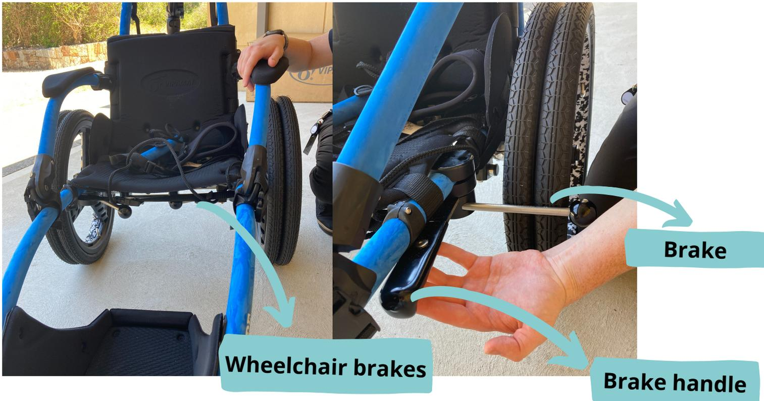
**Please note** brakes are designed to assist with transfers only. Brakes will not prevent the wheelchair from rolling down a steep hill.
