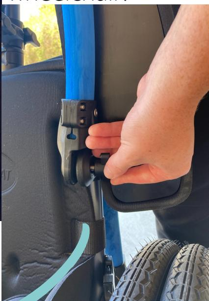
**Step 3.** To completely remove the armrest, unscrew the top bolt of the armrest. Remove the screw and fastening bolt. Place loose items in the storage box provided inside the shed.
