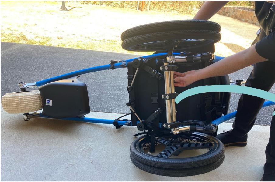
**Step 3.** To attach the new wheels, ensure the wheelchair is lying on its side.
