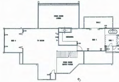
UPPER FLOOR - POWER LAYOUT A10 1:100
