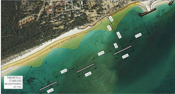
Above: PR1 Sand nourishment - Concept scheme (URS, 2012d) Left: PR3 Offshore Structures/breakwaters - Concept scheme (URS, 2012d) Figure 7.15 - MU3 Foreshore Reserve, Mu4 Southwest Foreshore Reserve And Toilet Block – Shortlisted Options PR1, PR3, PR4, PR7, PR9.
