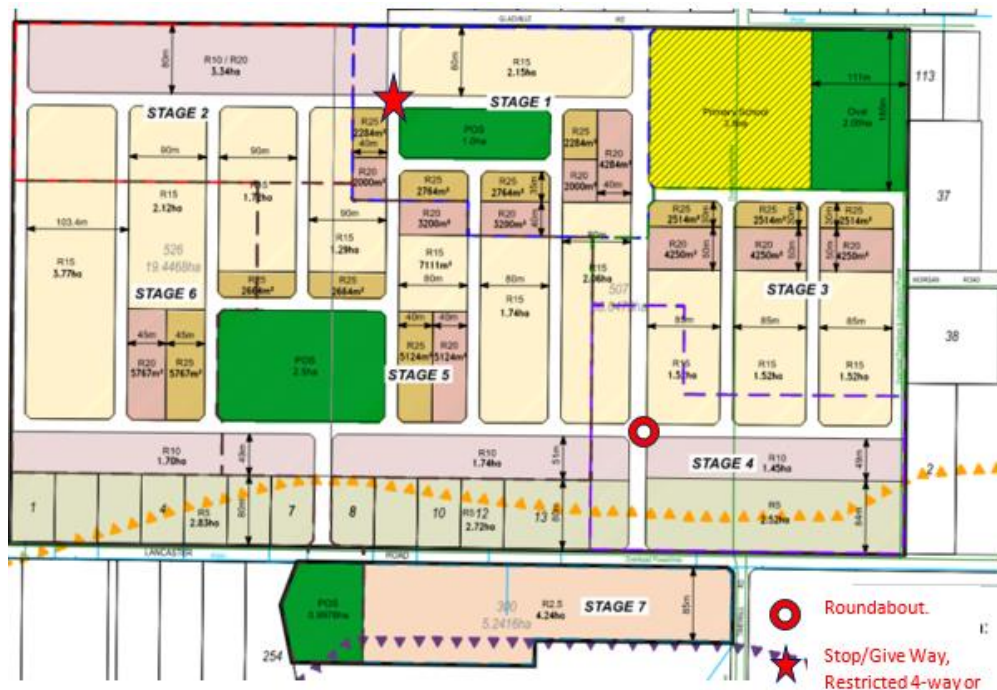
Figure 4-3: LSP Proposed Intersection Controls
