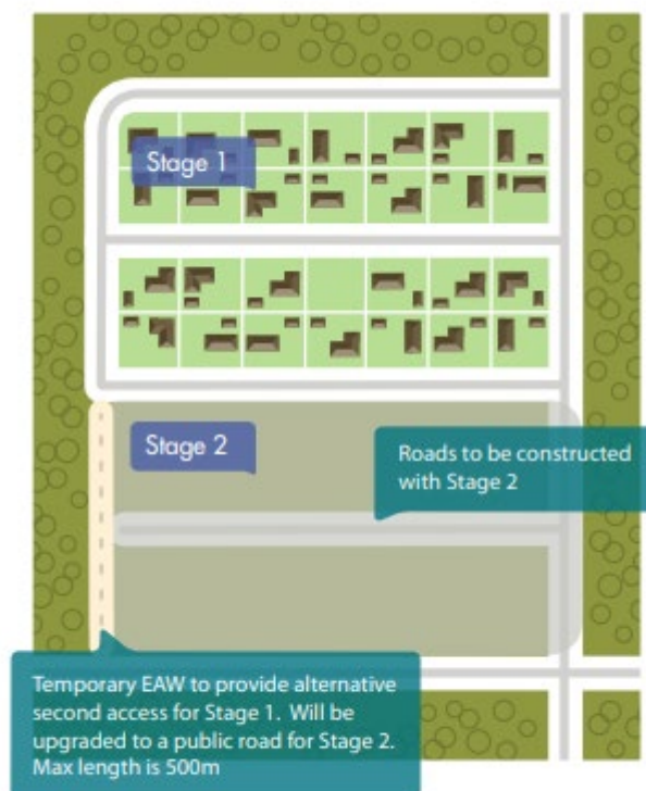
Figure 22: Example of an emergency access way
