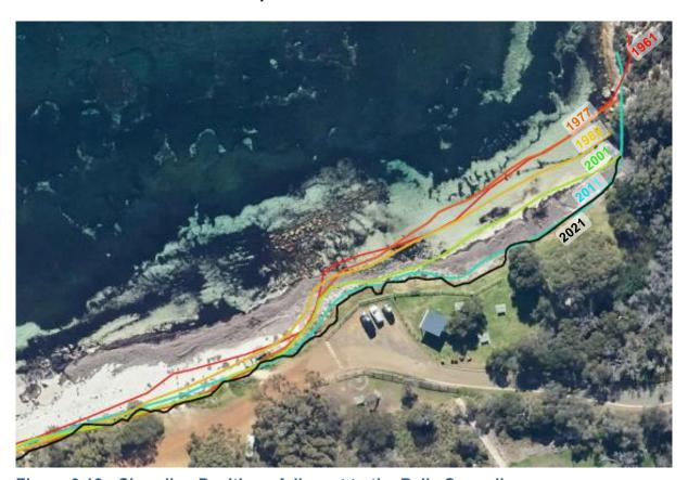
Figure 3.12 Shoreline Positions Adjacent to the Relic Seawall
