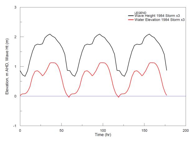
Figure 3.4 Storm Conditions for use in Storm Erosion Modelling (as determined for the area immediately offshore from the Resort site)
