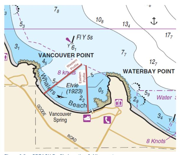
Figure 3.5 SBEACH Profile Location & Alignment
