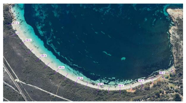
Figure 3.9 Intervals for Measurement of Shoreline Movement
