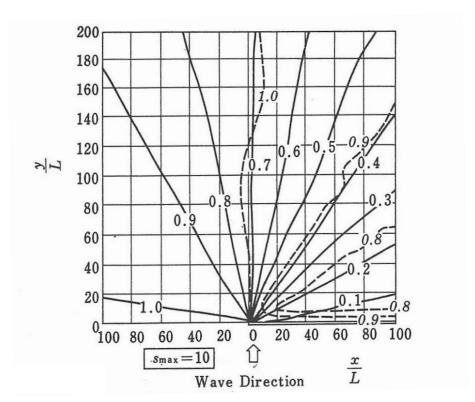
Figure 3.2 Diffraction Diagram from Goda (2010)
