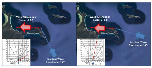
Figure 3.3 Examples of Wave Diffraction Attenuation Calculations
