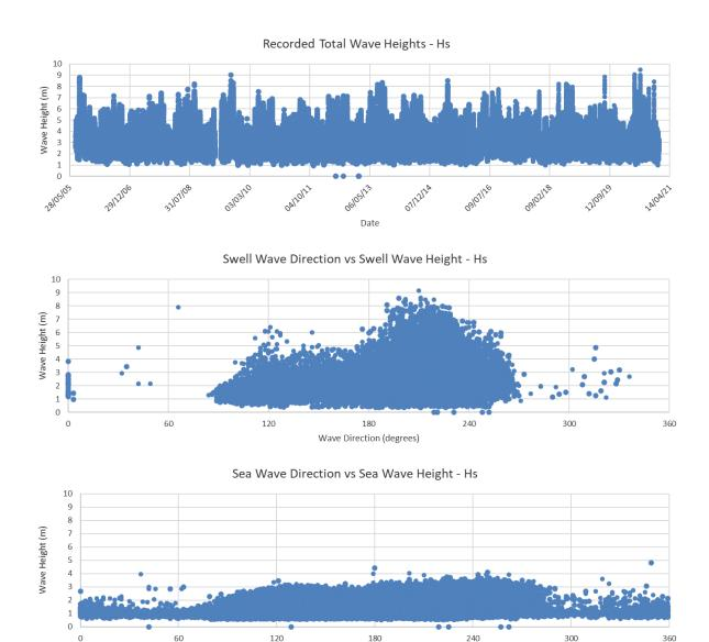
Figure 2.9 Wave Data Recorded from the Albany Waverider Buoy
