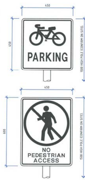
S9 CAR PARK SIGNAGE NON-ILLUMINATED ALUMINIUM REFLECTIVE SIGN ON GALVANISED STEEL POLE TYPICAL.
