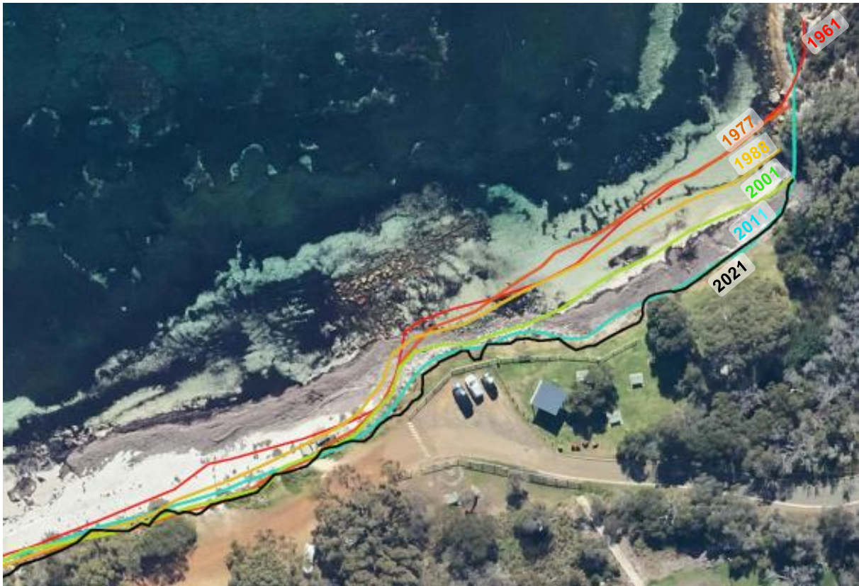
Figure 3.12 Shoreline Positions Adjacent to the Relic Seawall
