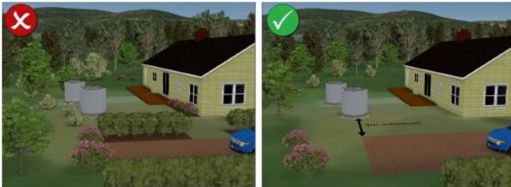
Figure 8: A good and a bad example of landscaping around a water tank and relation to hardstand areas. (WAPC, 2021)
