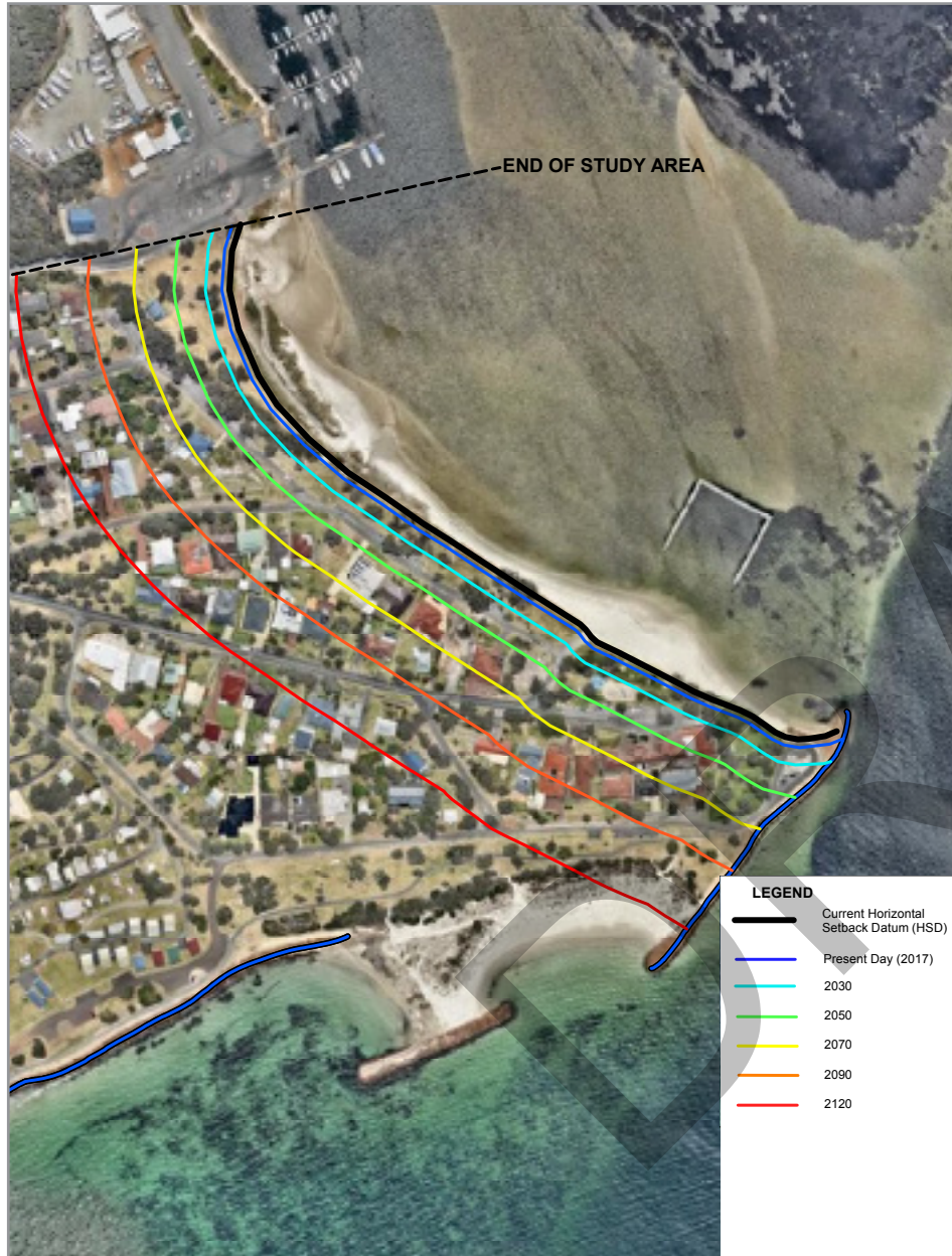
Figure 15 Emu Point to Middleton Beach Coastal Vulnerability with existing structures retained on the southern side of Emu Point
