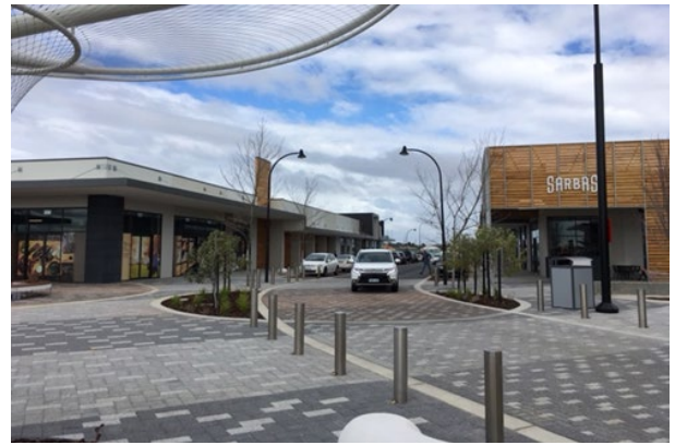
Design Guide – town centre main street with paving, bollards, lighting and landscape treatments to promote a slow-speed environment.
