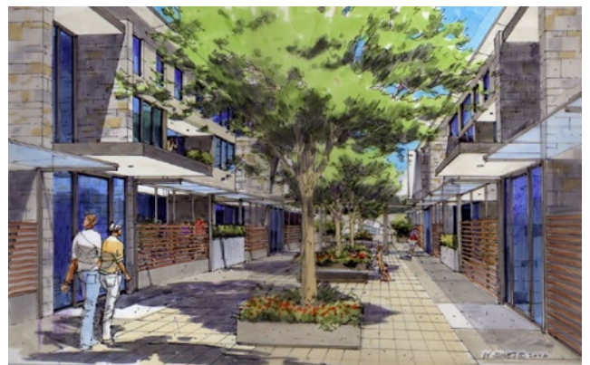
Design Guide – pedestrian access way framed with nil-boundary setback, ground floor development incorporating adaptability for future opportunity as commercial tenancies.
