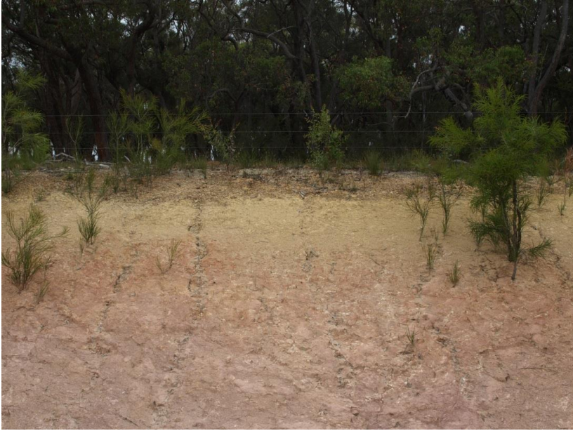
17. Exposed soil profile – roadside cutting along Down Road showing subsoil clay below gravel / laterite layer within upland terrain (U) land units.
