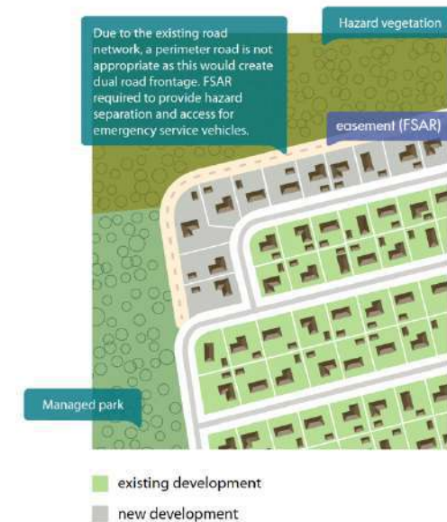
Example of Fire Service Access Way
