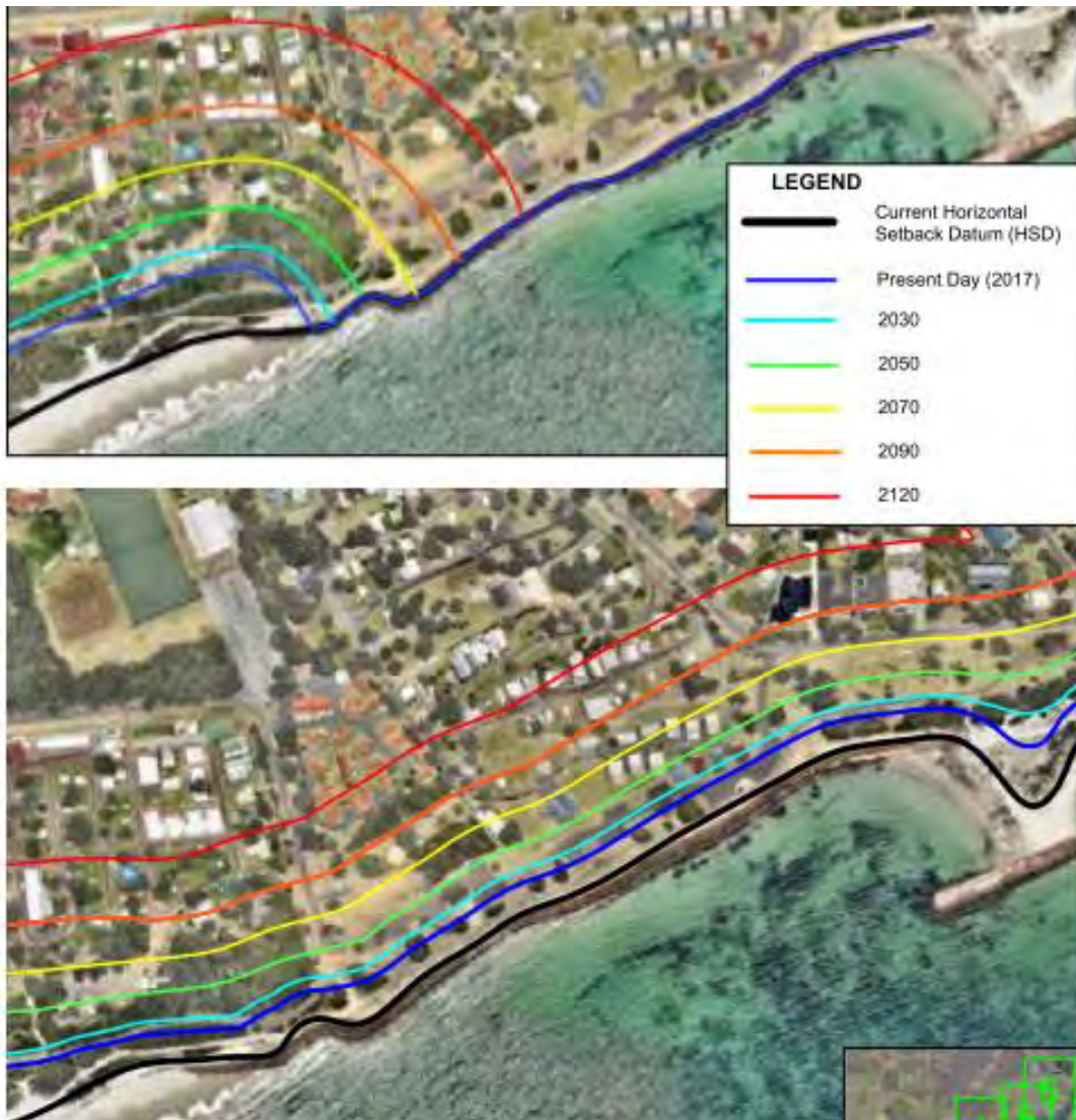
Figure 8: MU4 Hazard Map with existing structures (top) without existing structures (bottom). (Source: RHDHV, 2017).
