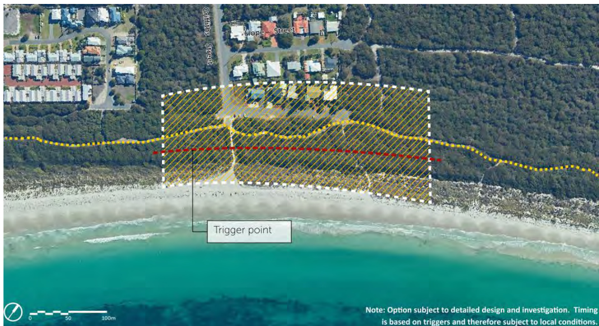
Figure 3: MU3 Griffiths Street Recommended Adaptation Option: Managed Retreat. Relocate properties from Griffiths Street
