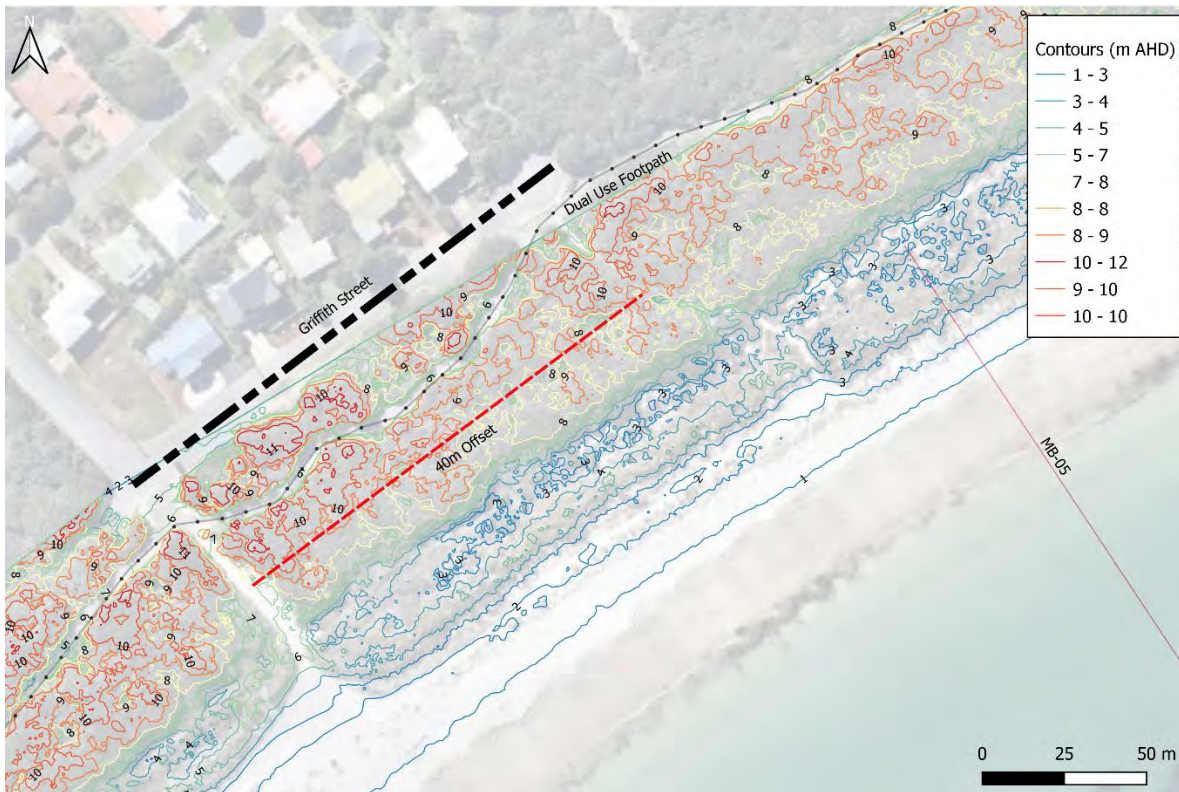
Figure 19: Contour map of the Griffiths Street foreshore from March 2019 showing the 40m seaward offset Coastal Adaptation Trigger Point and long-term beach transect MB-05
