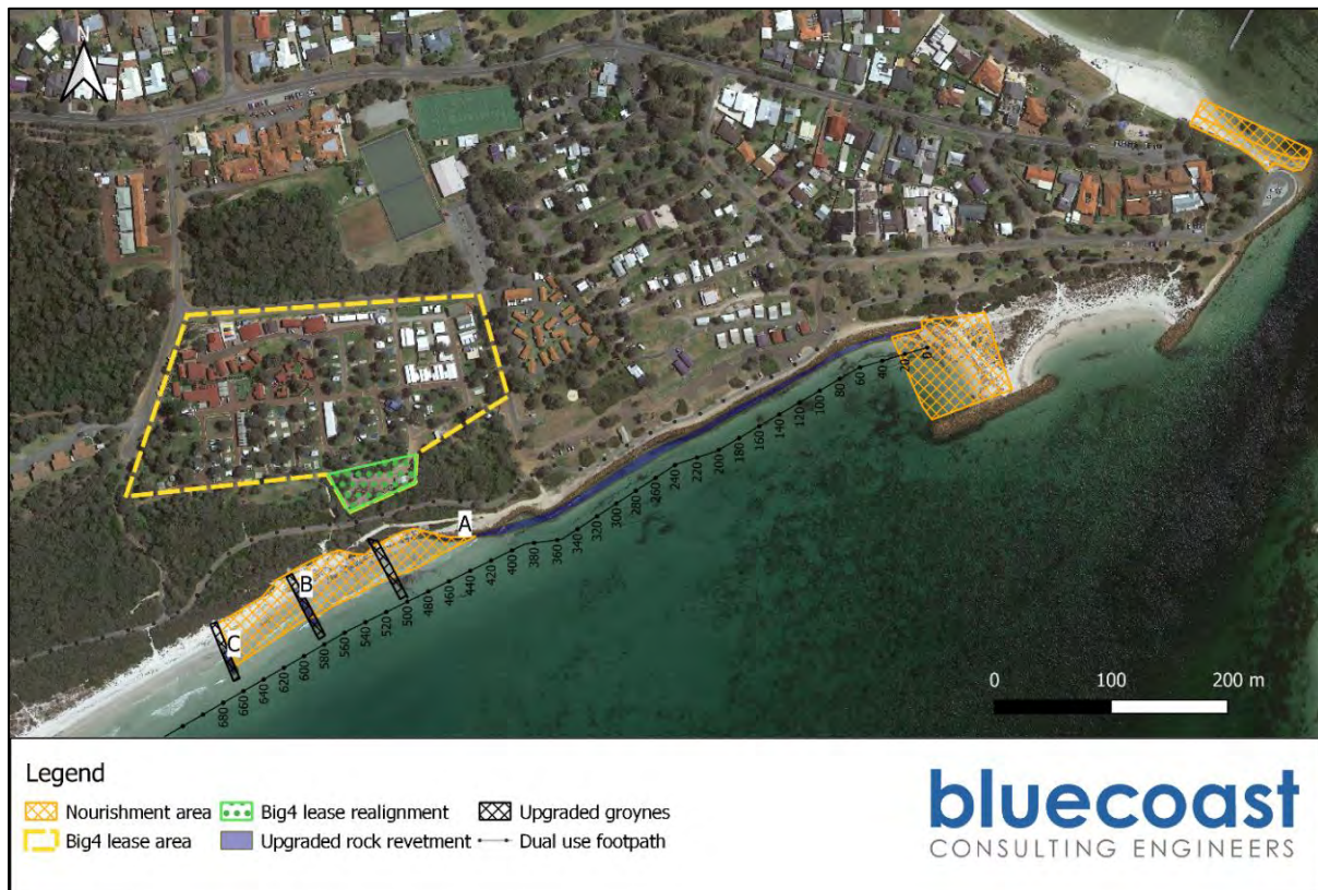
Figure 18: Coastal adaptation recommendations: rock revetment upgrade, upgrade of GSC trial groynes with beach nourishment and amendment of Big4 lease boundary.
