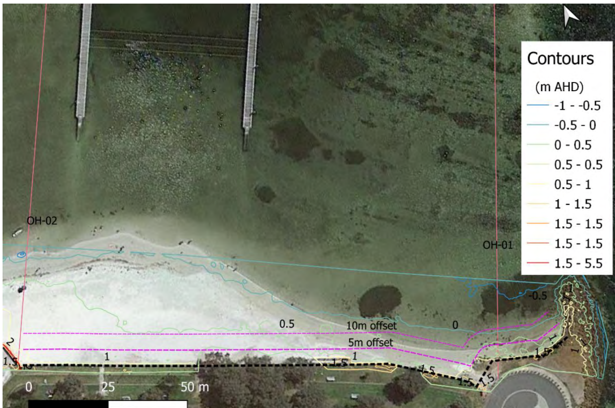
Figure 30: Contour map of eastern Oyster Harbour Beach. Beach transects OH-01 and OH-02 can be seen in red with the back beach hard revetment depicted by the black dashed line.
