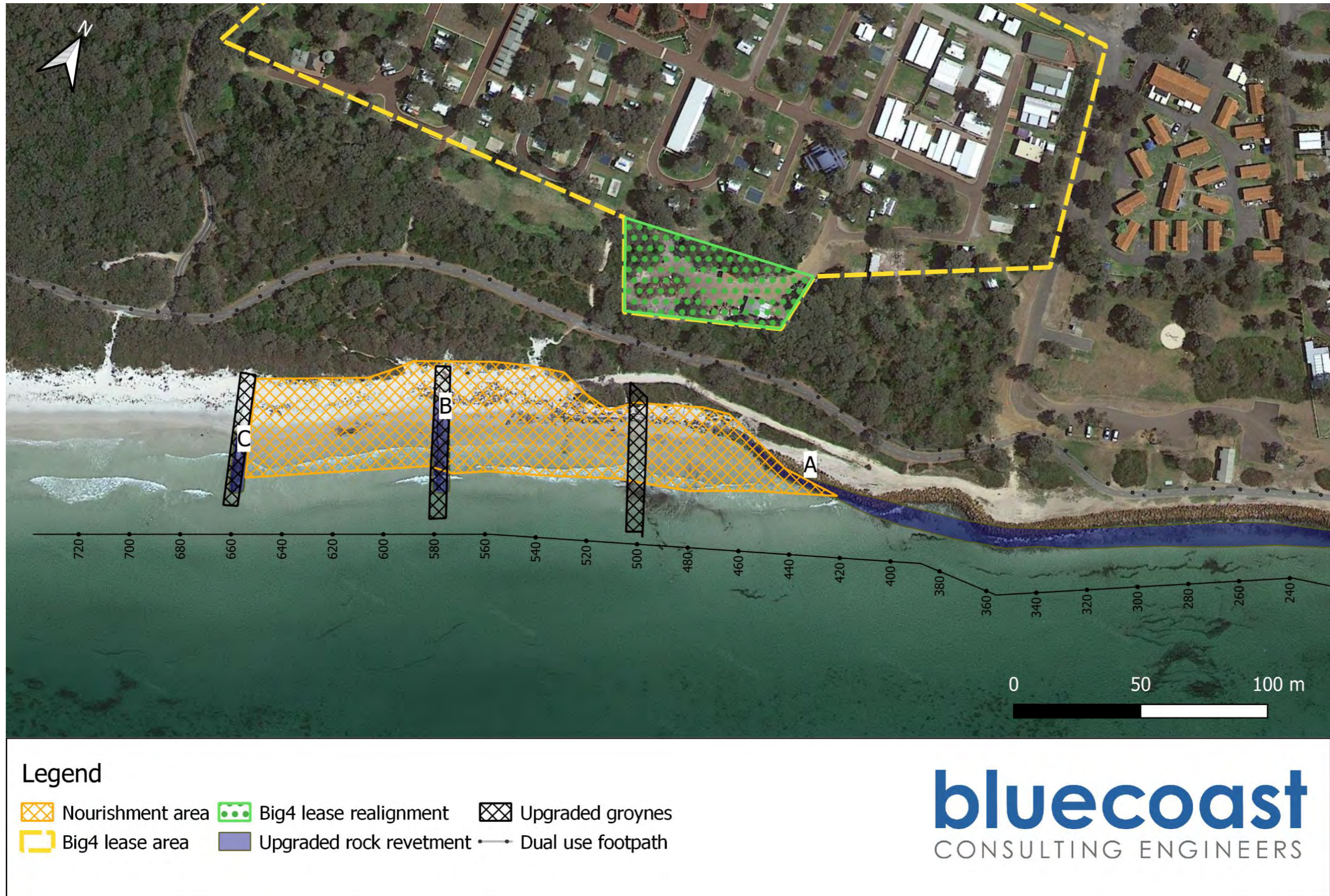
Figure 37: Coastal Adaptation Option: Groyne upgrade concept, Plan View
