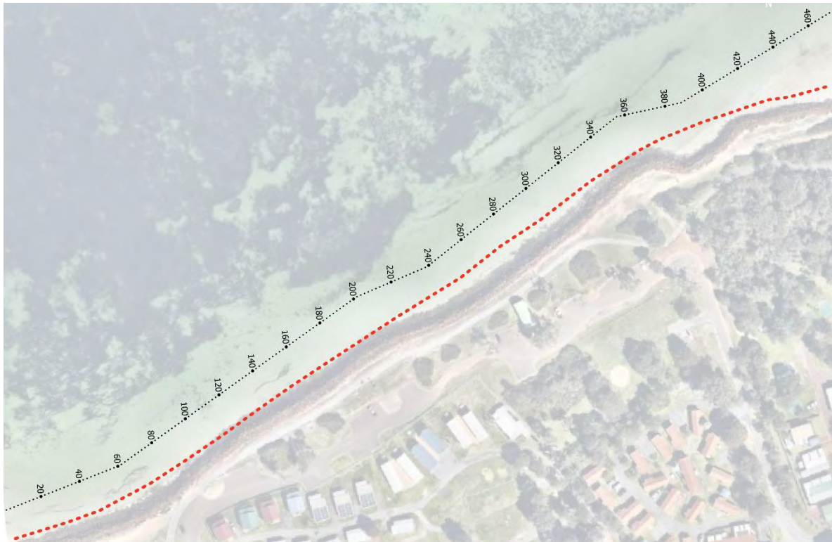
Figure 24: Current and proposed alignment of Coastal Structure A. The dotted red line represents the alignment of the rock revetment toe.
