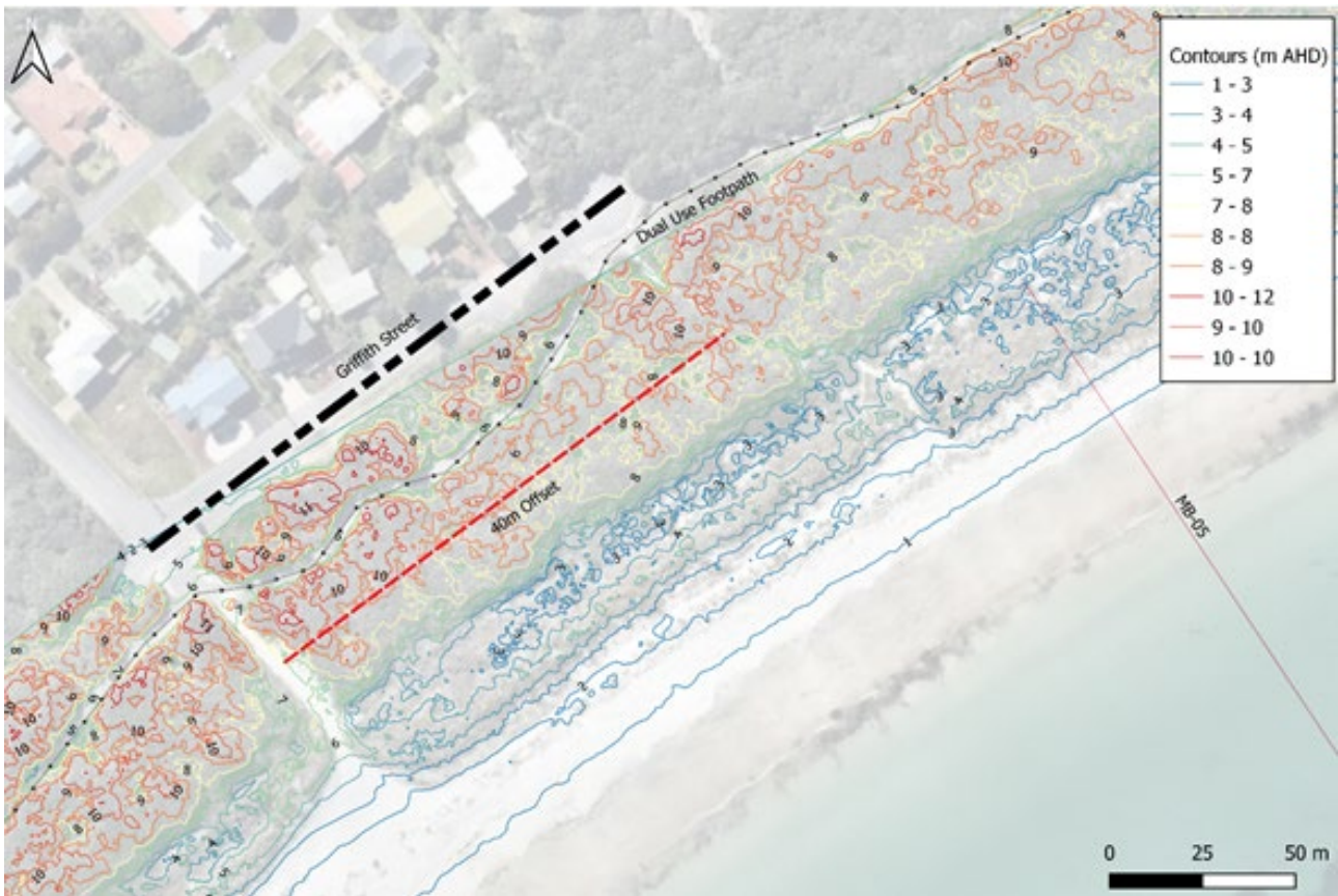
Figure 5: Topographic survey (March 2019) of the Griffiths Street foreshore and 40 m trigger value
