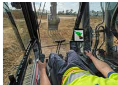
Dig Assist apps, powered by Volvo Co-Pilot
