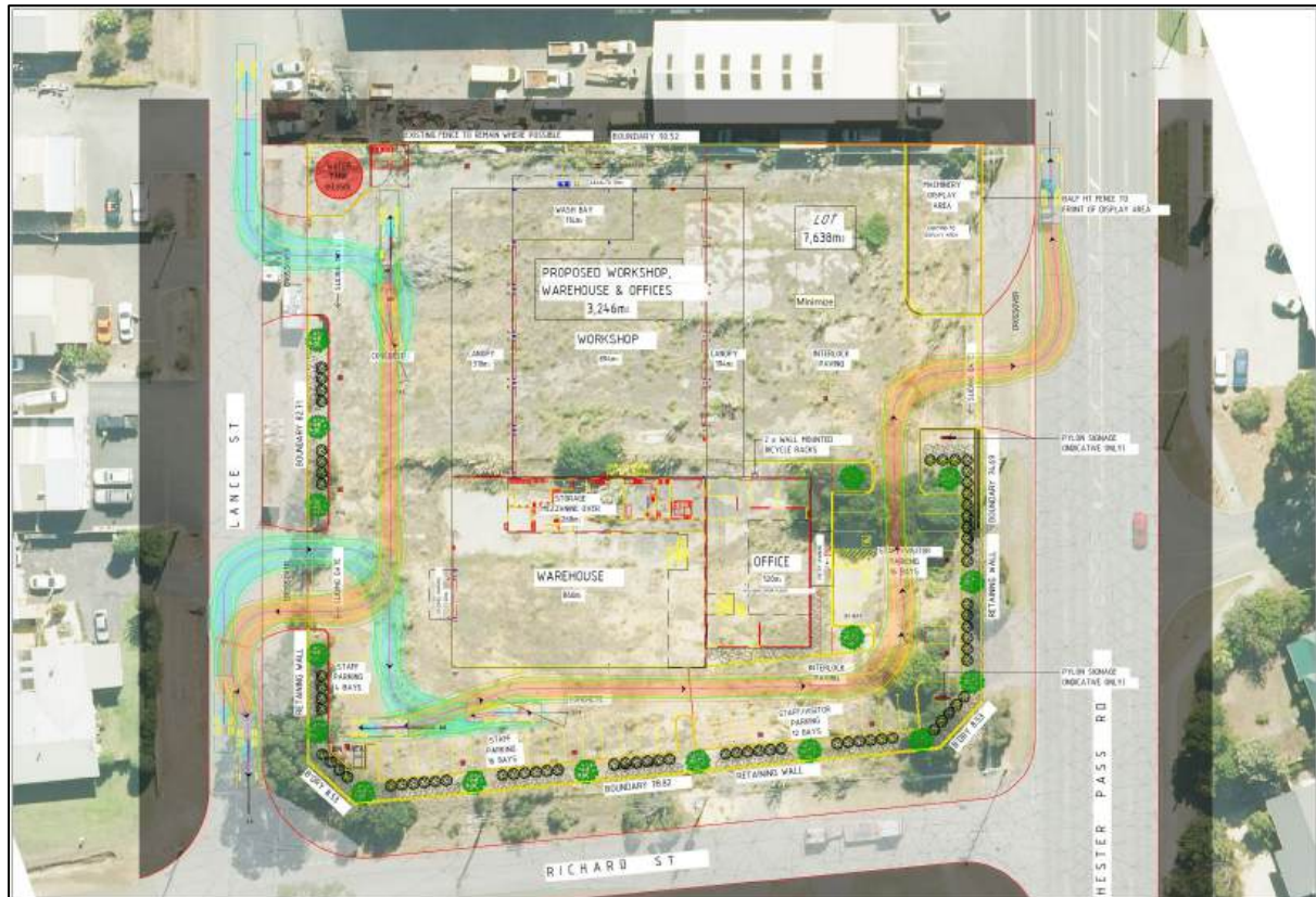
Figure 6 Swept Path – Waste Vehicle
