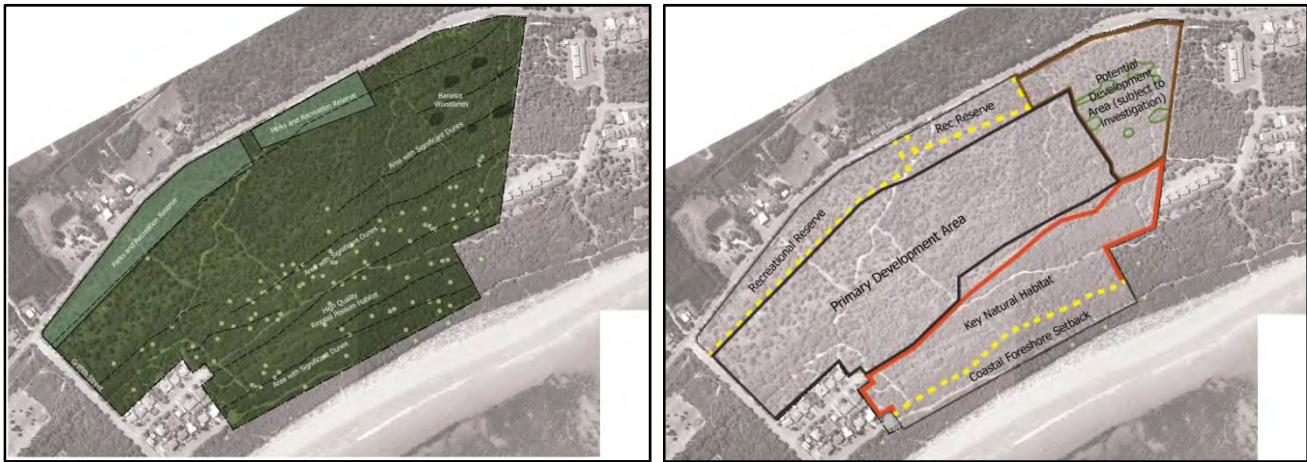
Figures 2.9 and 2.10: 2007 Site constraints assessment (left) and identification of primary development area (right).
