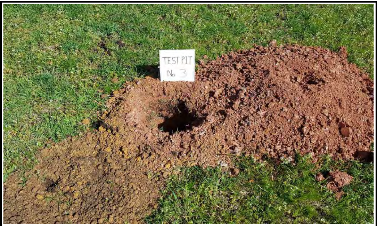
Test Pit No. 3 Spoil
