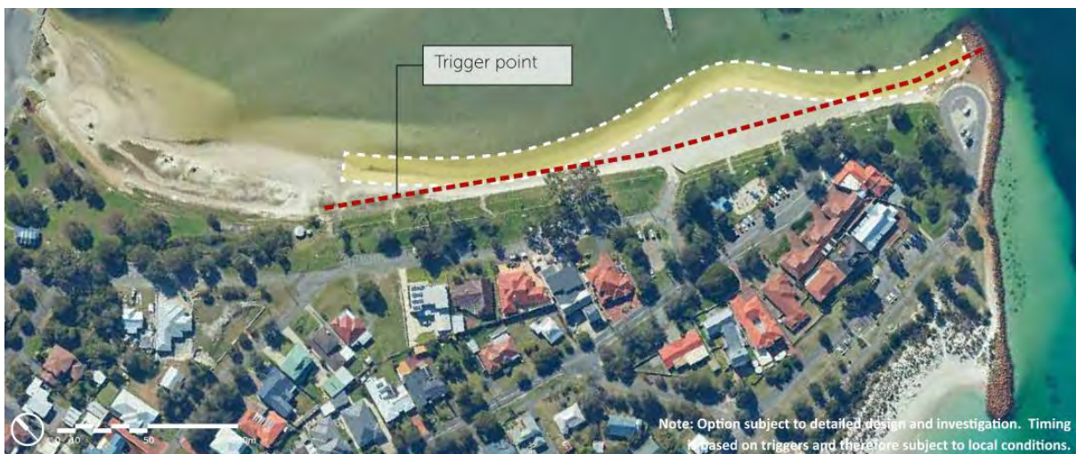
Figure 7: Recommendation 20: MU5 Oyster Harbour Beach - Sand Nourishment Eastern Oyster Harbour Beach (source: Aurora, 2019).
