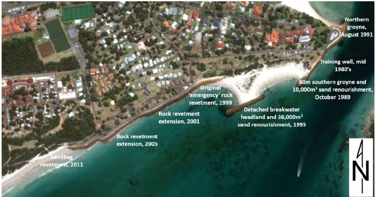
Figure 1: History of construction of coastal structures at Emu Point (source: RHDHV, 2017)
