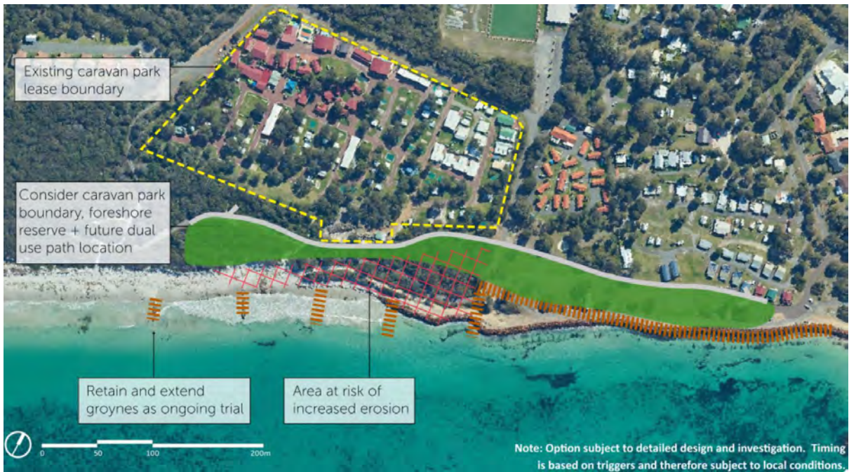
Figure 4: MU4 Emu Point Caravan Park CHRMAP recommendations 15: Emu Beach Holiday Park - Managed Retreat of assets in the southern portion and expansion of groynes (source: Aurora, 2019).
