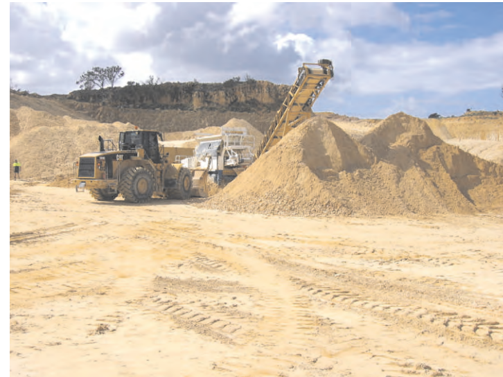
Loader feeding a small mobile crusher
