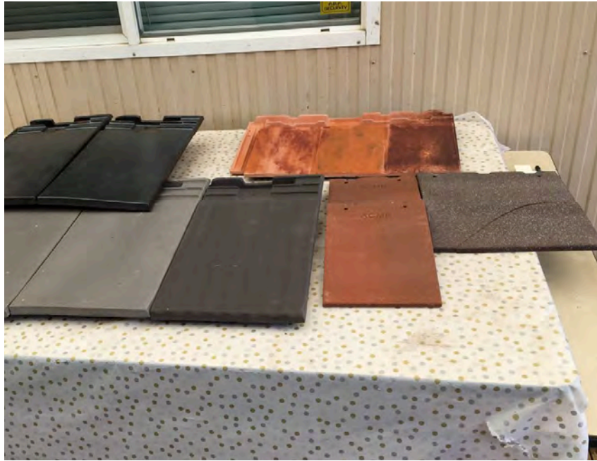
Photo 8 The Midland Brick Terracotta Shingle in Asphalt colour is in the centre of the photo, with the Marley Eternit Single Camber plain tile to the right
