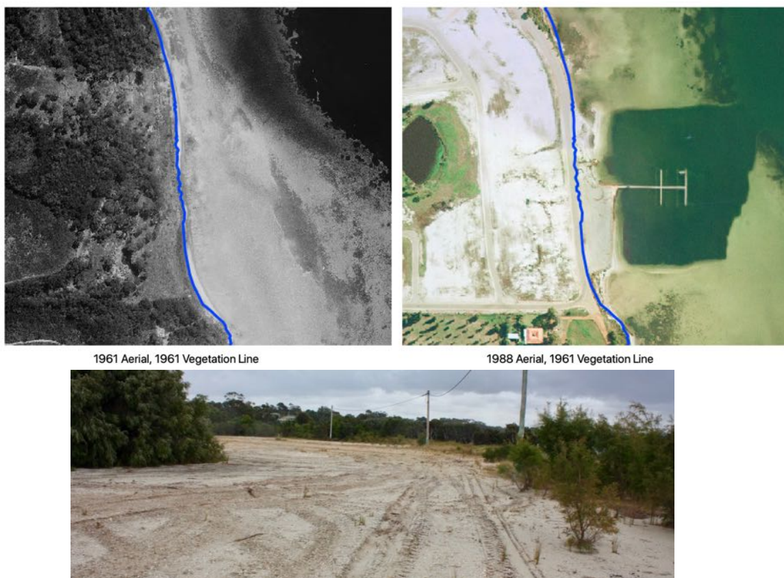
Figure 4.6 Lots 503 to 506 Windermere showing the change from 1961 (left) to 1988 (right), with the construction of the boat ramp and associated dredging, with shells evident on site during inspection (lower).
