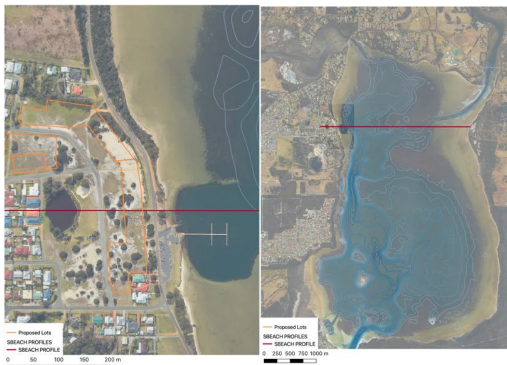
Figure 4.4 SBEACH modelled profile at Lower King showing path across proposed Lots (left), and extension through Oyster Harbour (right)
