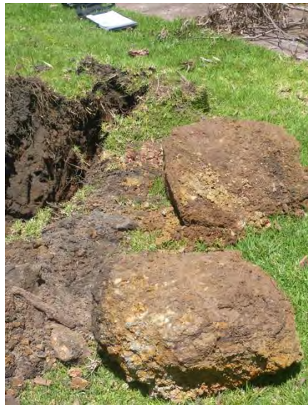
Photograph 4: Granite floaters from TP-C
