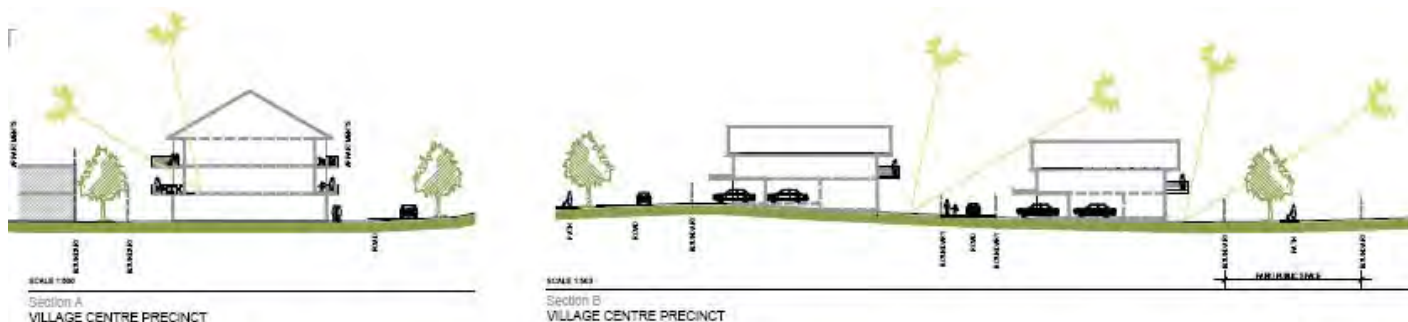
Figure 4.4 Cross sections of the Apartment and terrace buildings showing the vertical building envelopes (H+H Architects)
