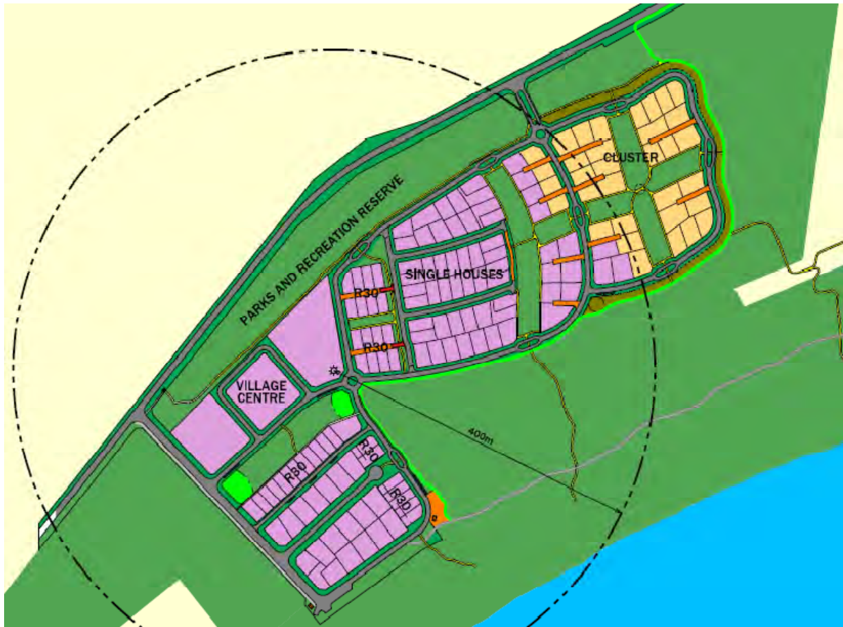
Figure 4.16: “Ped-Shed” to Village Centre
