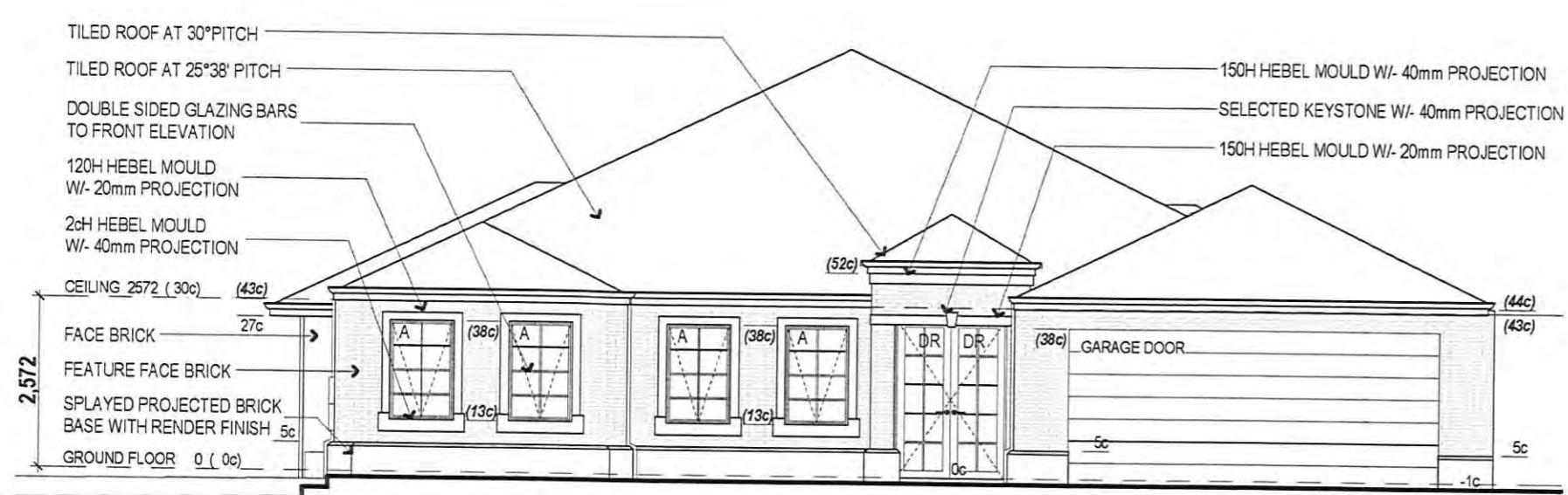
ELEVATION 1 (WEST) SCALE 1:100
