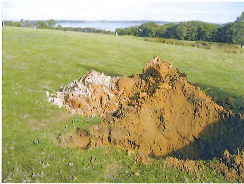
Test hole 2, showing well drained loam soils with high phosphate retention capability
