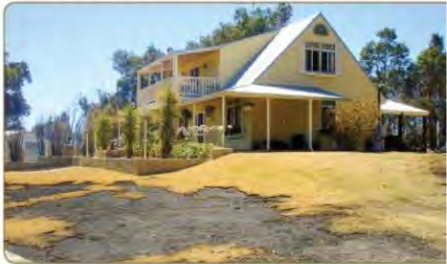
Above: Well prepared Building Protection Zone with reduced fuel.
