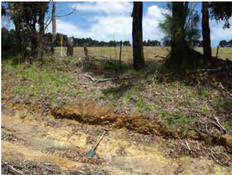
10. Land unit Sg2 Roadside cutting site 23 with gravel hardpan over clay subsoil
