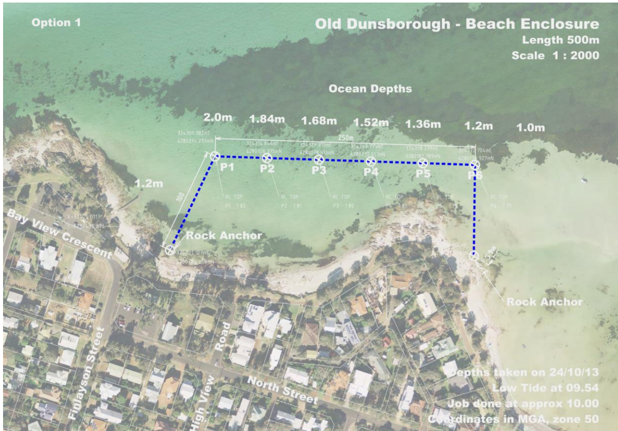
Figure 2-1 Design and layout of Dunsborough beach enclosure
