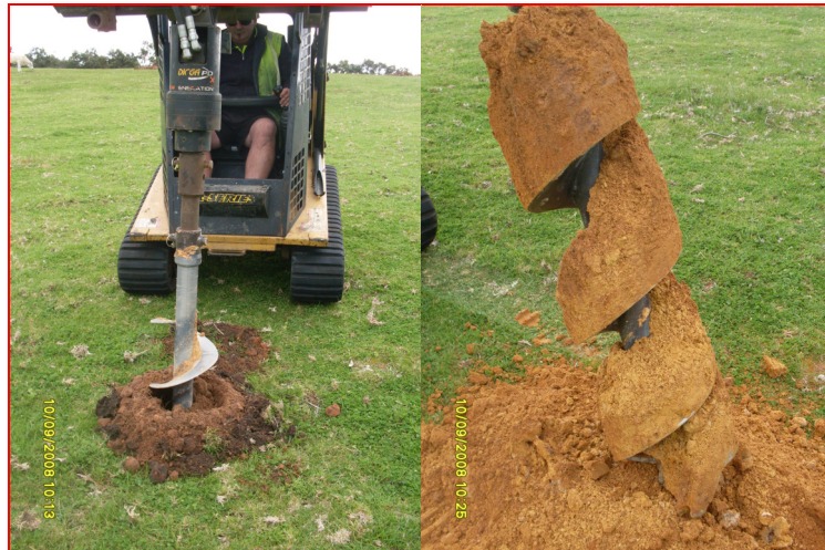
Plate 5: Test Pit 2 showing typical Map Unit B soils
