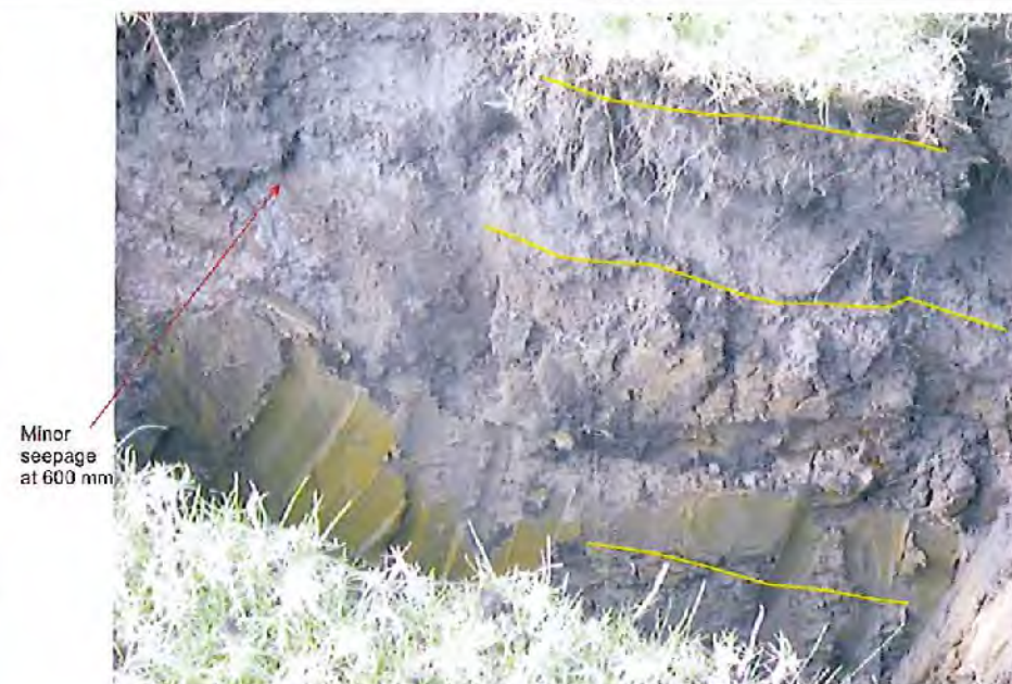
Test Hole 1, showing sand over yellow silt, with the layer of clay at the top of the silt subsoils. NOTE Clay has been spread deeper down the hole by the bucket.
