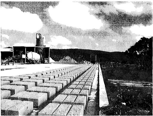
5. The blocks are stored on a gravel storage area adjacent to the concrete hardstand.
