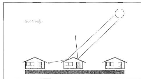
Figure 2: Modifying roof pitch or shielding to avoid directly reflected sunlight
