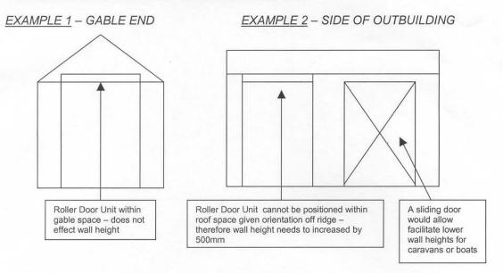
• It is not only the height of the caravan that needs to be considered, but the positioning of the openings. If the opening is located at the gable end the roller door unit, which is typically 500mm in height, can be accommodated within the roof space. Openings at the side of an outbuilding need to add 500mm to accommodate the roller door unit.
