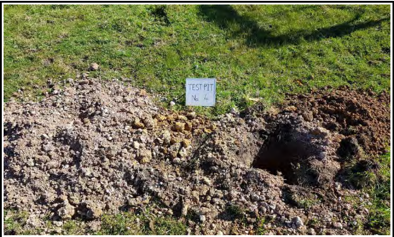
Test Pit No. 4 Spoil
