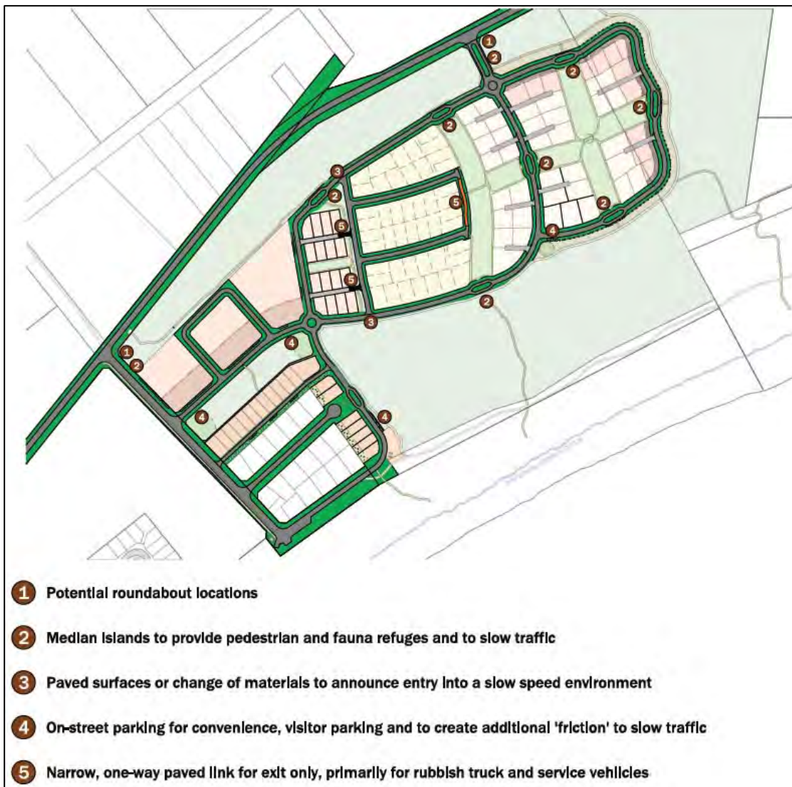
Figure 4.20 – Indicative Plan of traffic management measures to encourage a slow speed environment
