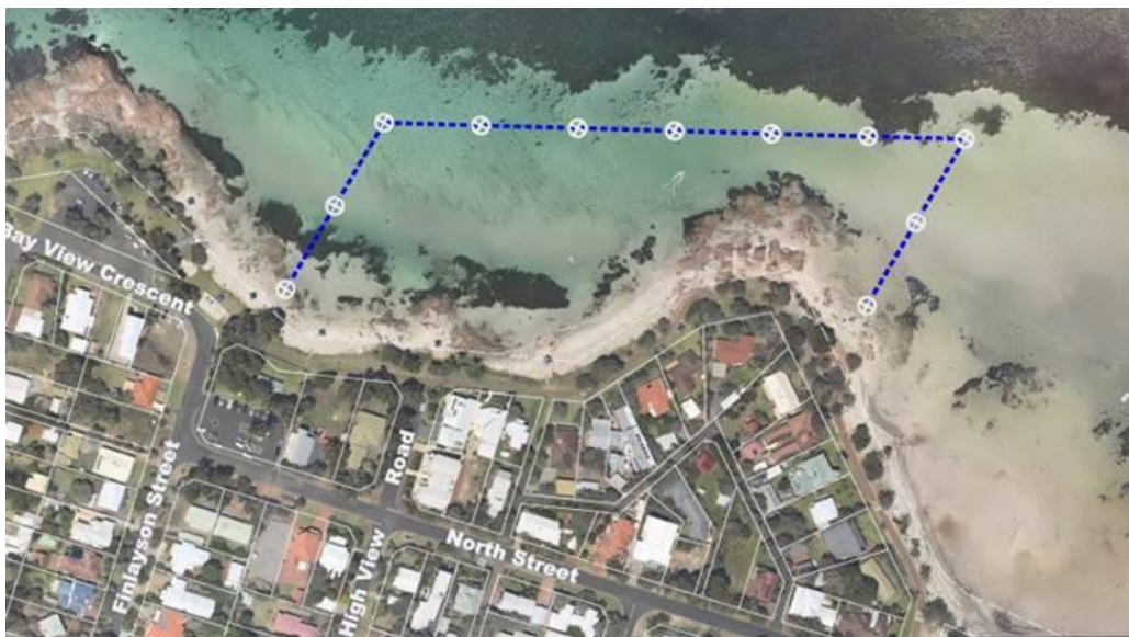
Figure 1-1 Dunsborough beach enclosure plan, designed to prevent sharks entering the designated area of water
