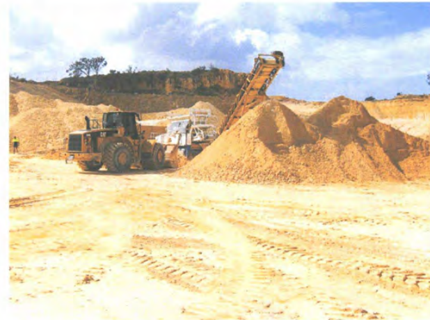
Loader feeding a small mobile crusher
