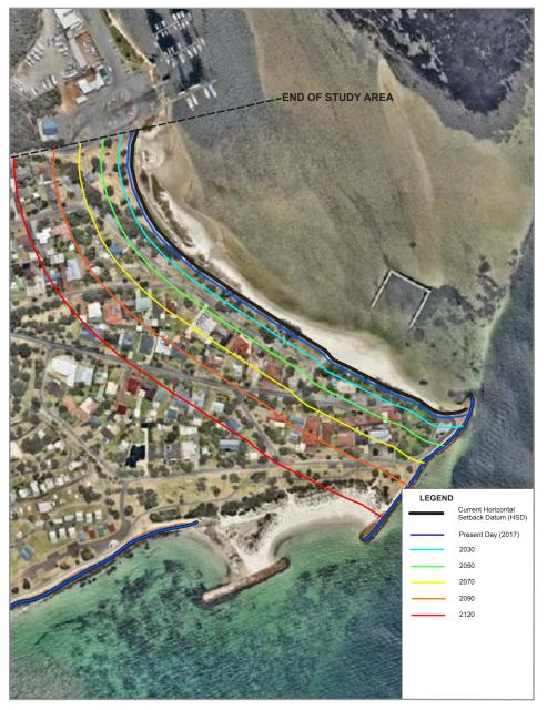
Figure 15 Emu Point to Middelton Beach Coastal Vulnerability with existing structures retained on the southern side of Emu Point
