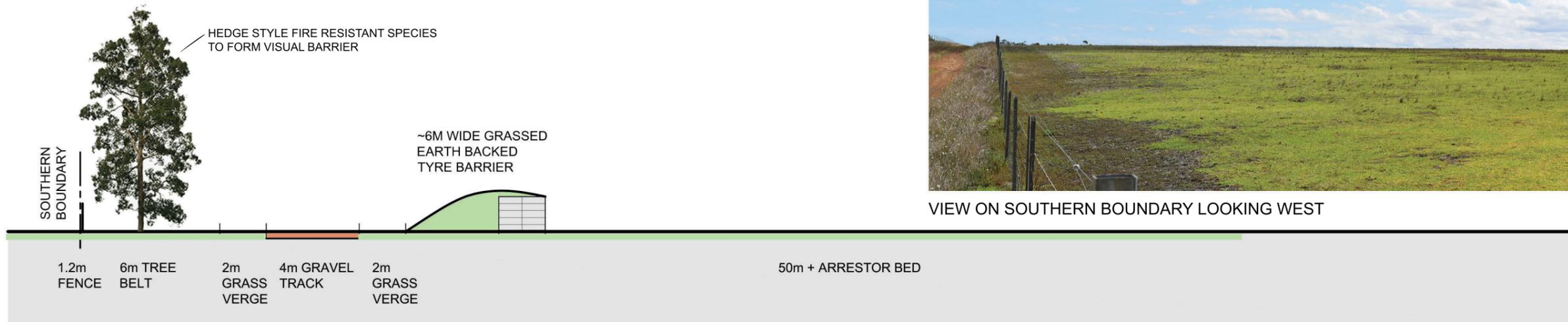
SECTION THRU SOUTHERN BOUNDARY (AT ARRESTOR BED)
