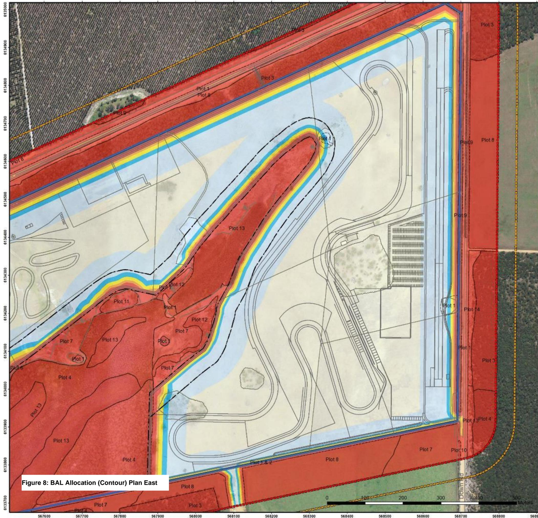
Figure 8: BAL Allocation (Contour) Plan East
