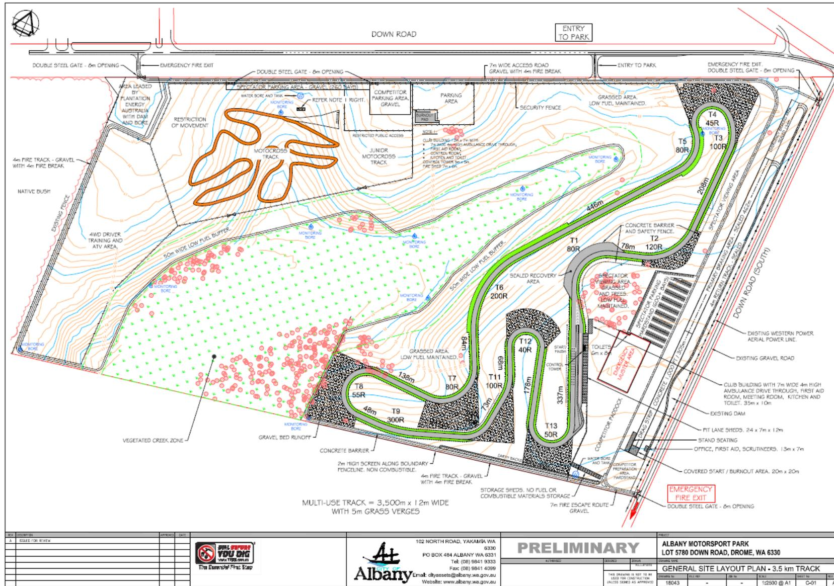
Figure 2: AMP General Site Layout Plan (Concept Plan)
