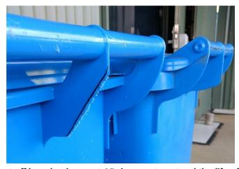
Centre rib cut off by a hacksaw at 45 degrees to extend the life of the bin lid.
