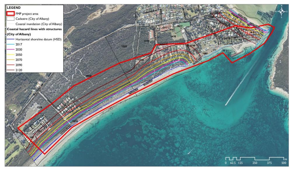
Figure 3: Coastal hazard risk for the FMP area over the 100 year planning period with coastal structures
