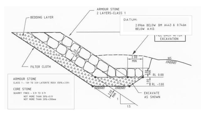
Figure 17: Emu Point Foreshore stabilisation revetment typical cross-section, May 2007 (Source: DoT, DWG 452-12-2)
