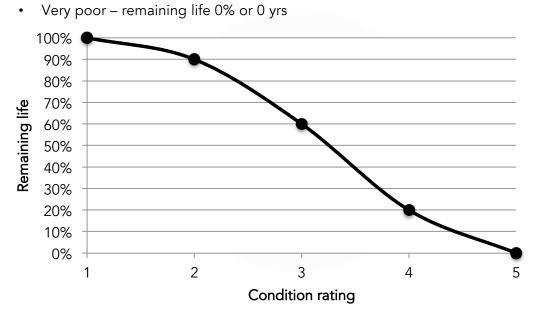
Figure 1. Remaining life relative to condition rating (1. very good, 2. good, 3, moderate, 4. poor, 5. very poor)
