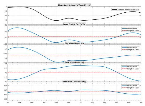
Figure 49: Mean longshore sediment transport potential at hindcast extraction point P3 after CERC (1984)
