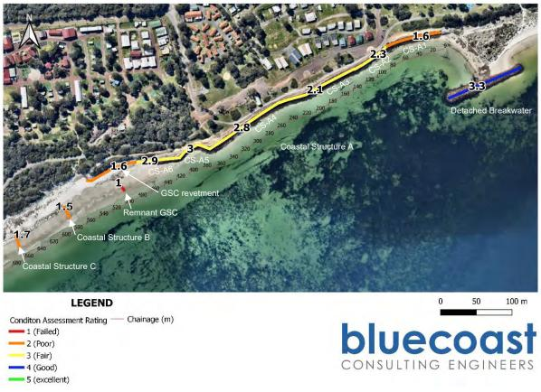
*Figure 2: Structure segments and crest chainage system defined for the existing structure as well as structural condition rating for structure based on visual and drone inspection on 26<sup>th</sup> February 2020.*
