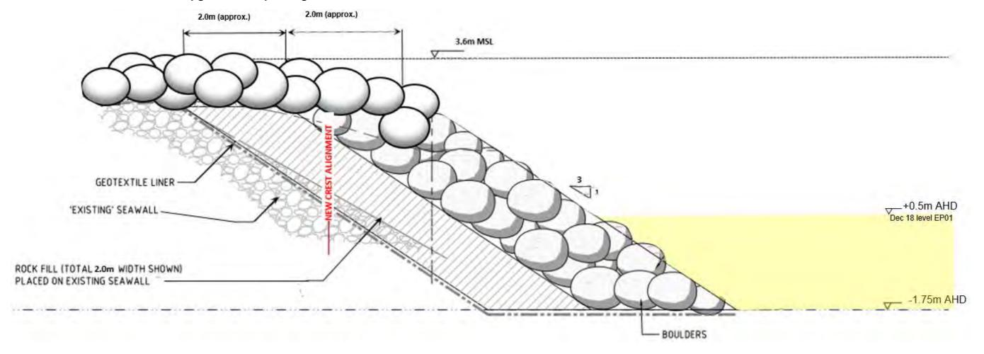
Figure 35: Coastal Adaptation Option 1: Rock revetment (Coastal Structure A) upgrade concept design. Please note all dimensions and levels are approximate and are to be confirmed during detailed design
