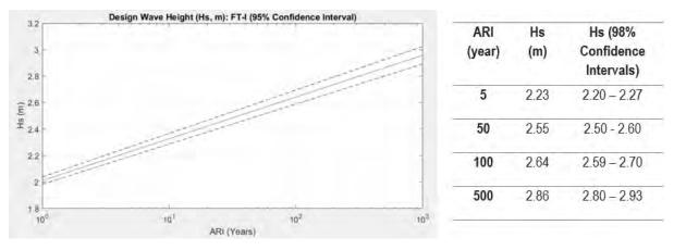
Figure 12: Design wave heights (H $_{\!s})$  from the central model extraction point (P2) from the 41 year hindcast wave model
