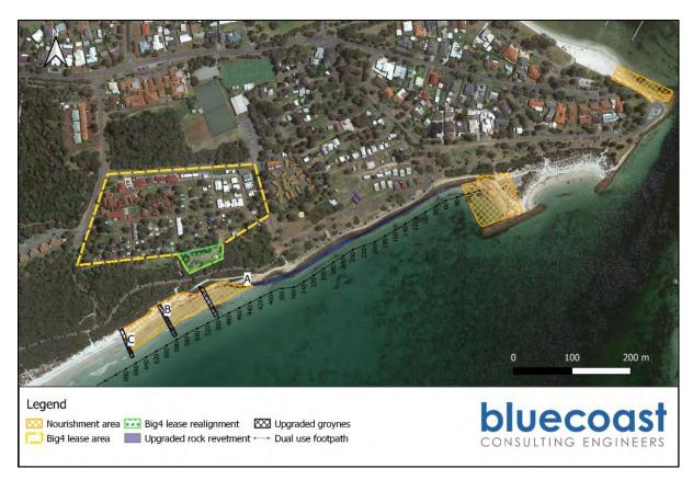
Figure 18: Coastal adaptation recommendations: rock revetment upgrade, upgrade of GSC trial groynes with beach nourishment and amendment of Big4 lease boundary.
