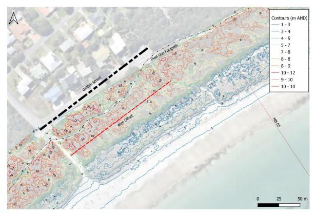
Figure 19: Contour map of the Griffiths Street foreshore from March 2019 showing the 40m seaward offset Coastal Adaptation Trigger Point and long-term beach transect MB-05 Note: These contours are taken form the March 2019 survey where contour heights within heavily vegetated areas represent the top of the vegetation.
