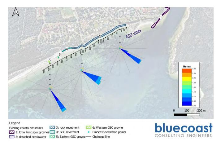
Figure 42: Long-term average wave roses from the three-model extraction point (P1, P2, P3) from the 41 year hindcast wave mode
