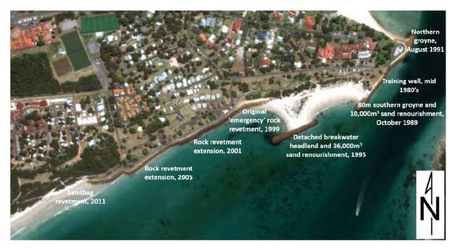
Figure 1: History of construction of coastal structures at Emu Point (source: RHDHV, 2017)
