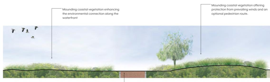
Dual use path (min 3m width) Secondary pedestrian path offering views along the coast. Flexible material (gravel) to limit maintenance in the event of over topping of the coastal structure.
