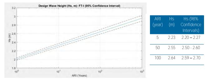
Figure 41: Design wave heights (H $_{s}$ ) of the central model extraction point (P2) from the 41 year hindcast wave model
