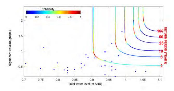
Figure 14: Bivariate return periods (RP) of water level and significant wave height.
