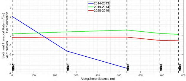
Figure 54: Sediment transport rates (m<sup>3</sup>/m) between MB-05 and MB-08 for the periods 2013 to 2014, 2014 to 2019 and 2019 to 2020. Note: erosion is negative.
