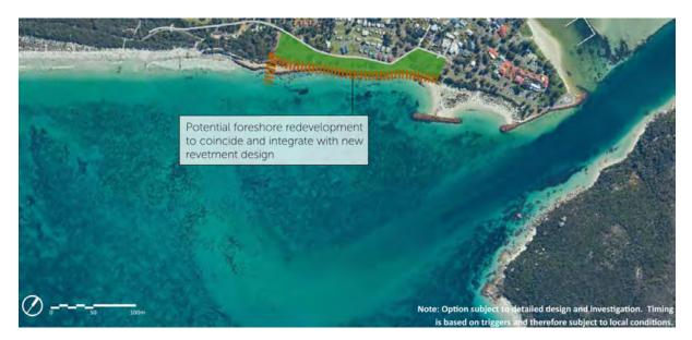
Figure 6: MU4 Foreshore Reserve CHRMAP recommendation19: Foreshore Reserve - Revetment be upgraded along with redevelopment of Foreshore park and removal of sandbag revetment (source: Aurora, 2019).
