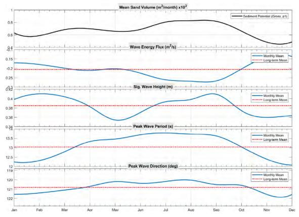
Figure 47: Mean longshore sediment transport potential at hindcast extraction point P1 after CERC (1984)
