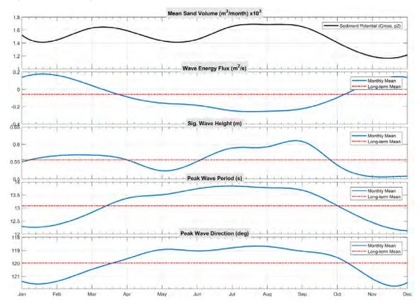
Figure 48: Mean longshore sediment transport potential at hindcast extraction point P2 after CERC (1984)
