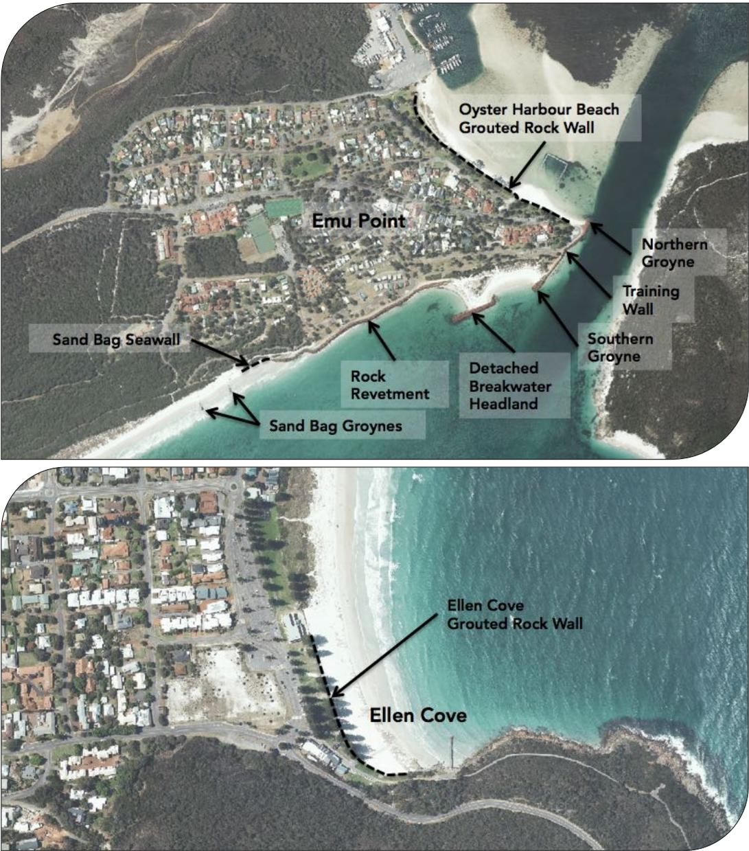
Figure 6. Coastal protection structure names MU4. Emu Point & MU1. Ellen Cove
