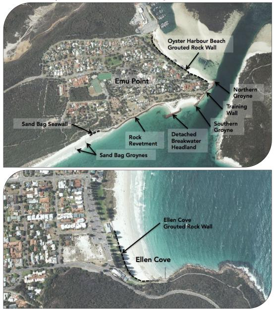
Figure 6. Coastal protection structure names MU4. Emu Point & MU1. Ellen Cove
